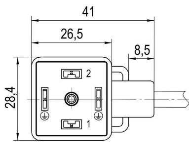
**Esquema de polos**
