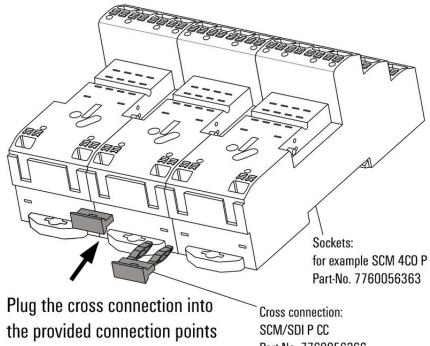
Plug the cross connection into the provided connection points
