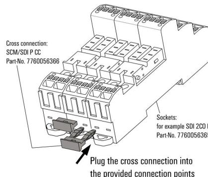
Plug the cross connection into the provided connection points
