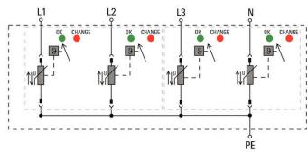
Schematic circuit diagram
