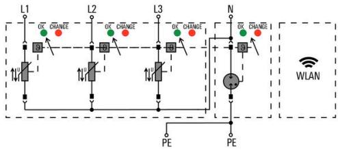
Schematic circuit diagram
