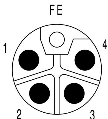
**Esquema de polos**
