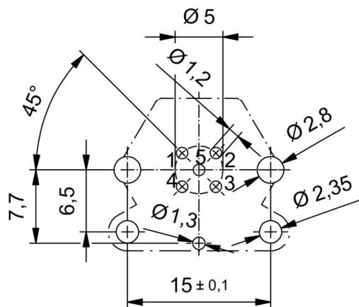
**Sección del panel frontal**
