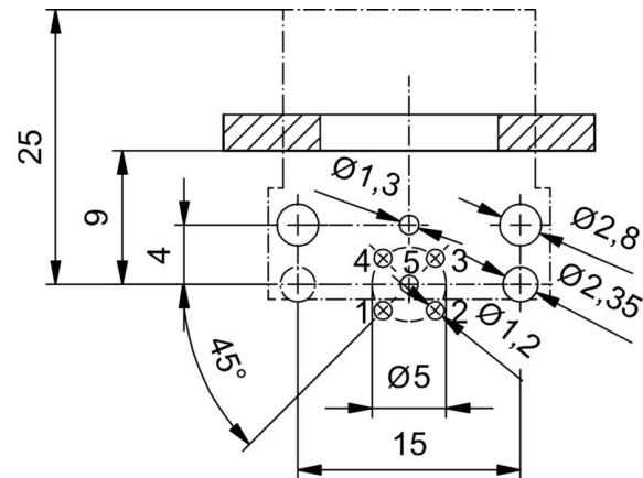
**Sección del panel frontal**
