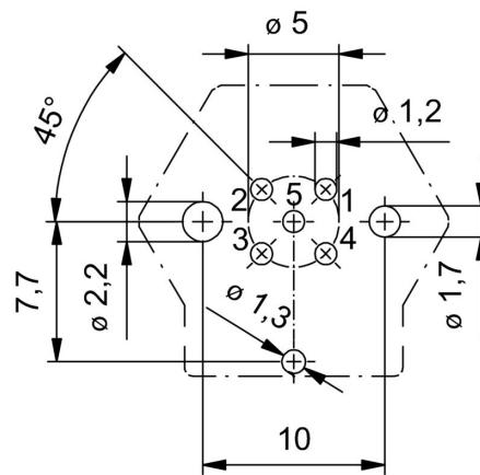
**Sección del panel frontal**
