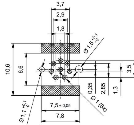
**Esquema de polos**
