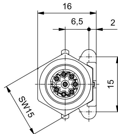
**Sección del panel frontal**
