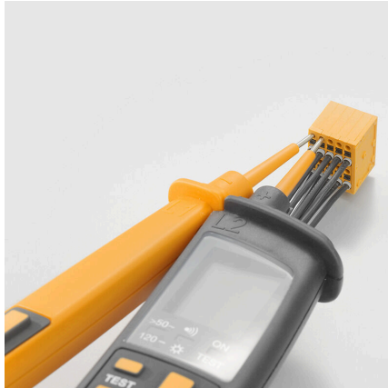
Maintenance through test tap
