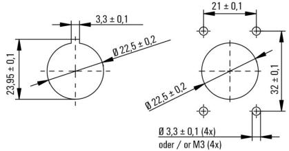
Mounting cut-out: 1. With central screw connection / 2. For mounting with four M3 screws
