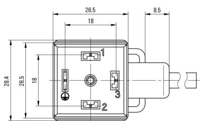
**Esquema de polos**
