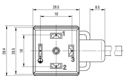
**Esquema de polos**
