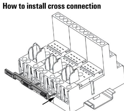
Plug the cross connection into wire-connection opening
