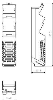
**Accesorios****CH20M AD SHL 5.00/04: tapa de elemento lateral para CH20M22, CH20M45, CH20M67**
