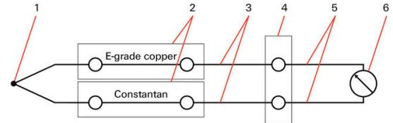
1. Thermocouple (sensor)
