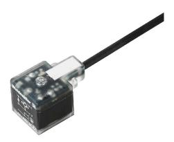
Weidmüller can supply valve plugs as connecting lines with M8/M12 plugs and one end without connector. The status of the valve plug is shown by an LED. The valve plugs have a protective circuit. The Weidmüller range includes valve plugs of type A, B and C to DIN and industry standards. Protection class IP 67 is fulfilled when screwed in. The outlet direction is also a decisive factor, therefore Weidmüller offers different versions.
