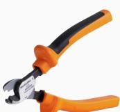
Cutting tools for conductors up to 8 mm, 12 mm, 14 mm and 22 mm outside diameter. The special blade geometry allows pinch-free cutting of copper and aluminium conductors with minimum physical effort. The cutting tools (KT 8 to KT 22) also come with VDE and GS-tested protective insulation up to 1,000 V in accordance with EN/IEC 60900.
