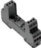
Base element for the pluggable VSPC arresters. Integrated PE foot in the base of the impedance-neutral VSPC BASE and floating earth PE connection (FG) via integrated sparkover gap, safely discharges up to 20 kA (8/20 µs) and 2.5 kA (10/350 µs) to PE. Suitable for unearthing signal circuits.
