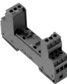
Base element for the pluggable VSPC arrester, integrated PE foot in impedance-neutral VSPC BASE. Can safely discharge up to 20 kA (8/20 µs) and 2.5 kA (10/350 µs) to the PE.
