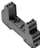
Base element for the pluggable VSPC arrester, integrated PE foot in impedance-neutral VSPC BASE. Can safely discharge up to 20 kA (8/20 µs) and 2.5 kA (10/350 µs) to the PE.
