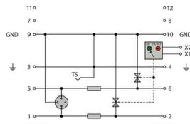
Complete module direct grounding, with remote signalling
