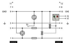
Complete module indirect grounding, with remote signalling
