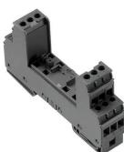
Base element for the pluggable VSPC arresters. Integrated PE foot in the base of the impedance-neutral VSPC BASE and floating earth PE connection (FG) via integrated sparkover gap, safely discharges up to 20 kA (8/20  $\mu$ s) and 2.5 kA (10/350  $\mu$ s) to PE. Suitable for unearthing signal circuits.
