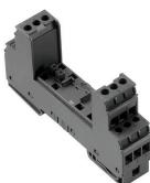
Base element for the pluggable VSPC arrester, integrated PE foot in impedance-neutral VSPC BASE. Can safely discharge up to 20 kA (8/20  $\mu$ s) and 2.5 kA (10/350  $\mu$ s) to the PE.
