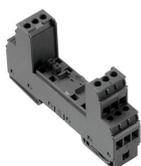
Base element for the pluggable VSPC arresters. Integrated PE foot in the base of the impedance-neutral VSPC BASE and floating earth PE connection (FG) via integrated sparkover gap, safely discharges up to 20 kA (8/20  $\mu$ s) and 2.5 kA (10/350  $\mu$ s) to PE. Suitable for unearthened signal circuits.
