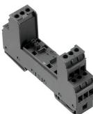
Base element for the pluggable VSPC arresters. Integrated PE foot in the base of the impedance-neutral VSPC BASE and floating earth PE connection (FG) via integrated sparkover gap, safely discharges up to 20 kA (8/20 µs) and 2.5 kA (10/350 µs) to PE. Suitable for unearthing signal circuits.
