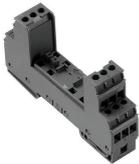
Base element for the pluggable VSPC arresters. Integrated PE foot in the base of the impedance-neutral VSPC BASE and floating earth PE connection (FG) via integrated sparkover gap, safely discharges up to 20 kA (8/20  $\mu$ s) and 2.5 kA (10/350  $\mu$ s) to PE. Suitable for unearthed signal circuits.
