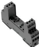
Base element for the pluggable VSPC arrester, integrated PE foot in impedance-neutral VSPC BASE. Can safely discharge up to 20 kA (8/20 µs) and 2.5 kA (10/350 µs) to the PE.
