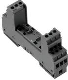
Base element for the pluggable VSPC arrester, integrated PE foot in impedance-neutral VSPC BASE. Can safely discharge up to 20 kA (8/20  $\mu$ s) and 2.5 kA (10/350  $\mu$ s) to the PE.
