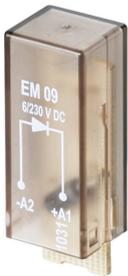
Pluggable protective modules for the RIDERSERIES RCI / RCM relay sockets, with optional protective functions.
