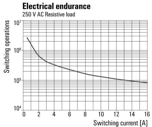
Electrical service life 250 V AC resistive load
