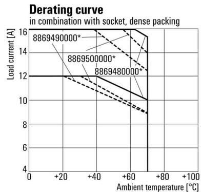
\* For full continuous current (16 A), the wire terminals 11 with 21, 12 with 22 and 14 with 24 must be bridged with a wire  $\geq 1,5 \text{ mm}^2$  at the socket.
