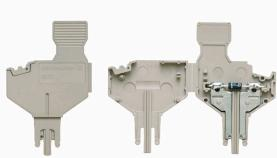
The component plug is used to integrate an electrical component in a disconnect terminal block. After soldering the electronic component, the plug can be integrated into the disconnection area of our disconnect terminal blocks and thus changes the disconnect terminal block into a modular terminal block with integrated electronic component.
