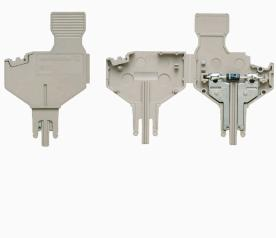
The component plug is used to integrate an electrical component in a disconnect terminal block. After soldering the electronic component, the plug can be integrated into the disconnection area of our disconnect terminal blocks and thus changes the disconnect terminal block into a modular terminal block with integrated electronic component.
