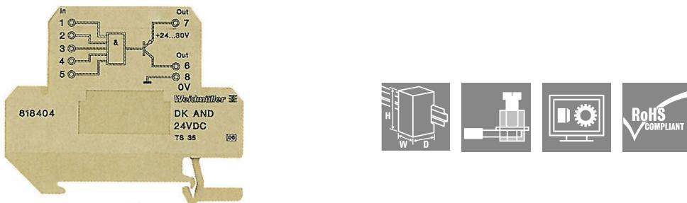
Logic functions AND, NAND, OR and NOR in modular terminal format with a rated cross-section of 4 mm<sup>2</sup>. They each have five inputs which are fed – with logic gating – via a 24 V/20 mA PNP output. The logic components can be used for many applications involving the coupling of digital sensor/actuator signals with automation devices.
