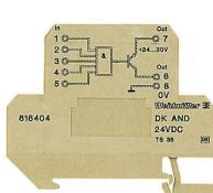
Logic functions AND, NAND, OR and NOR in modular terminal format with a rated cross-section of 4 mm<sup>2</sup>. They each have five inputs which are fed – with logic gating – via a 24 V/20 mA PNP output. The logic components can be used for many applications involving the coupling of digital sensor/actuator signals with automation devices.
