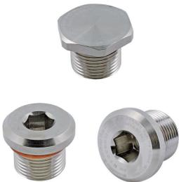
VP series stopping plugs provide a method of filling unused entries in Ex equipment while maintaining Flameproof Ex d and Increased Safety Ex e explosion protection and IP66/67/68 ingress rate.
