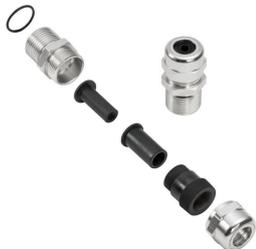
Brass cable glands which are suitable for usage in explosion risk zone Ex e (Increased safety). They have been tested to the latest norms and standards IEC/EN 60079-0, and also achieved the necessary ATEX certificate.
