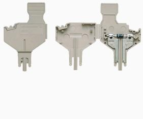
The component plug is used to integrate an electrical component in a disconnect terminal block. After soldering the electronic component, the plug can be integrated into the disconnection area of our disconnect terminal blocks and thus changes the disconnect terminal block into a modular terminal block with integrated electronic component.
