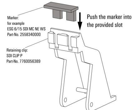
How to install marker on retaining clip
