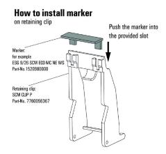
How to install markeron retaining clip
