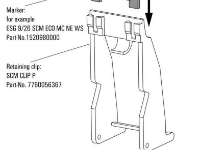
How to install marker on retaining clip
