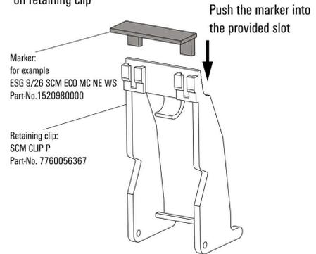
How to install marker on retaining clip
