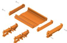
The RS 80 profile offers you a wide range of mounting options, as both mounting rail and wall mounting are possible. This allows flexible adaptation to your spatial conditions and requirements. For particularly heavy components, additional locking feet can be used to improve stability. Another advantage of the RS80 profile is that it can be individually cut to size. This gives you the freedom to design the system exactly according to your needs.
