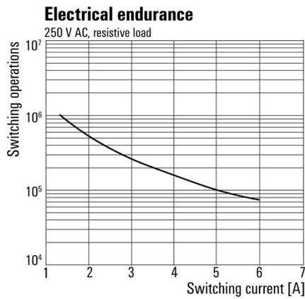
Electrical service life 230 V AC resistive load
