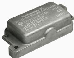
The option of separating cables in Zone 2 that comply with the following approvals ATEX: T II 3G Ex ec IIC T6 Gc or IECEx: Ex ec IIC T6 Gc simplifies installation, service and enables better preparation. The approved connectors offered here must always be used complete with the corresponding approved housings and inserts and may only be disconnected without load.
