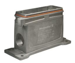
The option of separating cables in Zone 2 that comply with the following approvals ATEX: T II 3G Ex ec IIC T6 Gc or IECEX: Ex ec IIC T6 Gc simplifies installation, service and enables better preparation. The approved connectors offered here must always be used complete with the corresponding approved housings and inserts and may only be disconnected without load.
