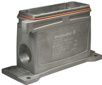
The option of separating cables in Zone 2 that comply with the following approvals ATEX: T II 3G Ex ec IIC T6 Gc or IECEx: Ex ec IIC T6 Gc simplifies installation, service and enables better preparation. The approved connectors offered here must always be used complete with the corresponding approved housings and inserts and may only be disconnected without load.
