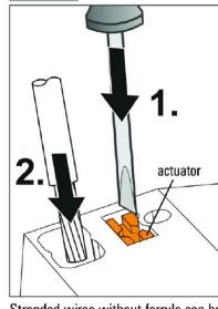
Stranded wires without ferrule can be inserted by pushing down the actuator using a screwdriver.
