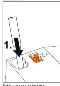
Solid wires can be inserted without opening the terminal.
