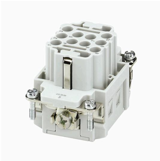
The HEE series features high-density contacts and is designed based on the established HE inserts. The wire connection level is designed as a PUSH IN contact. Number of poles: 10 - 64. Rated current: 16 A. Rated voltage: 500 V.
