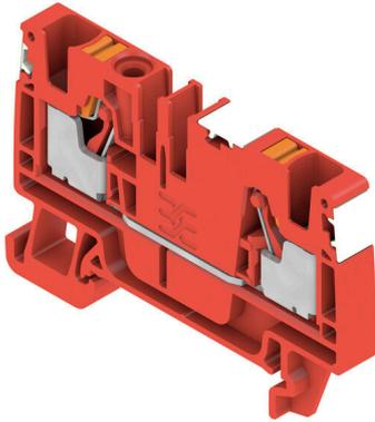
To feed through power, signal, and data is the classical requirement in electrical engineering and panel building. The insulating material, the connection system and the design of the terminal blocks are the differentiating features. A feed-through terminal block is suitable for joining and/or connecting one or more conductors. They could have one or more connection levels that are on the same potential or insulated against one another.
