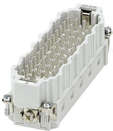
The HEE series features high-density contacts and is designed based on the established HE inserts. The wire connection level is designed as a PUSH IN contact. Number of poles: 10 - 64
