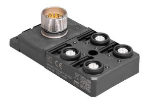
Whereas the standard M12 system requires the sleeves to be laboriously screwed on and that operation is hindered by the vibration guard, M12 Push-Pull works with one click, just like those well-known garden hose systems. The audible locking function guarantees a safe and reliable connection as well as a good seal. The new SAI M12 Push-Pull distributors can be used with M12 plug-in connectors but also with the new M12 Push-Pull plug-in connectors.
