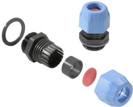
Polyamide cable glands, which are suitable for usage in explosion risk zones Ex e (increased safety) and Ex i (intrinsic safety). Weidmüller offers a product family without restrictions and besides compliance with standards, the cable gland excels thanks to its increased impact resistance of 4/7 Joule and a possible temperature range down to -60°C without restrictions. They have been tested to the current standard and EN 60079-0 directive, they are ATEX and IECEx certified.
