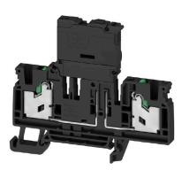
In some applications it is useful to protect the feed through connection with a separate fuse. Fuse terminal blocks are made up of one terminal block bottom section with a fuse insertion carrier. The fuses vary from pivoting fuse levers and pluggable fuse holders to screwable closures and flat plug-in fuses.
