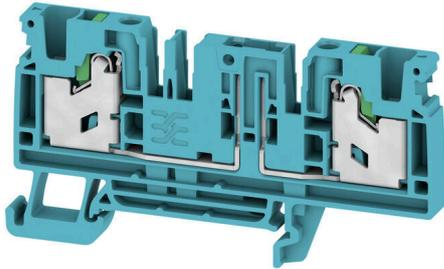
In some applications it makes sense to add a test point or a disconnect element to the feed through terminal for testing and safety purposes. With test disconnect terminals you measure electric circuits in the absence of voltage. While the disconnecting points clearance and creepage distance is not assessed in dimensional terms, the specified rated impulse voltage strength must be proven.
