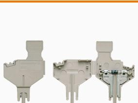
The component plug is used to integrate an electrical component in a disconnect terminal block. After soldering the electronic component, the plug can be integrated into the disconnection area of our disconnect terminal blocks and thus changes the disconnect terminal block into a modular terminal block with integrated electronic component.
